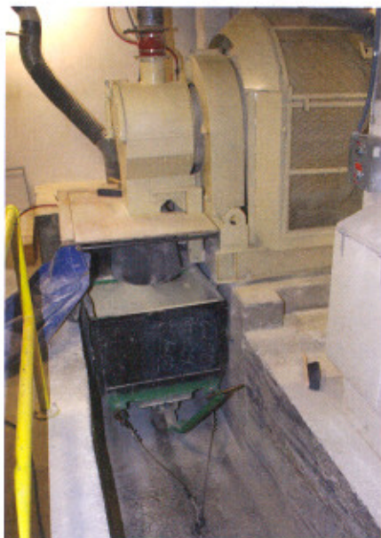
▲ The batch is rapidly discharged from the mixer into a cart that transports it to the furnace.
