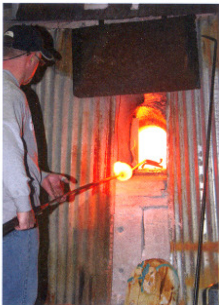
▲ The gatherer uses a punty, which is continually turned, to accumulate molten glass from the pot, and transfer it to a mould.
